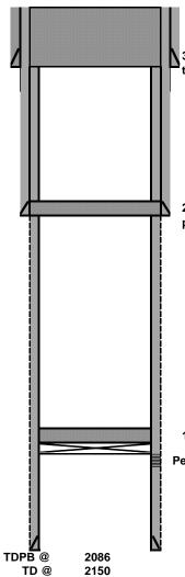
13 3/8 48# CSG @ 209 3. Perf'd @ 269'. Pressured up on perfs to 500 PSI. Spotted 45 sx class C cmt @ 400' to surface.
