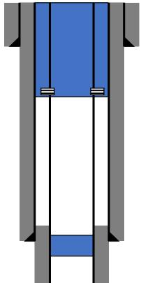
PERF @ 1300'. EST CIRC. CIRC 240 SX CL C CMT TO SURFACE. VERIFIED CMT @ SURFACE.
