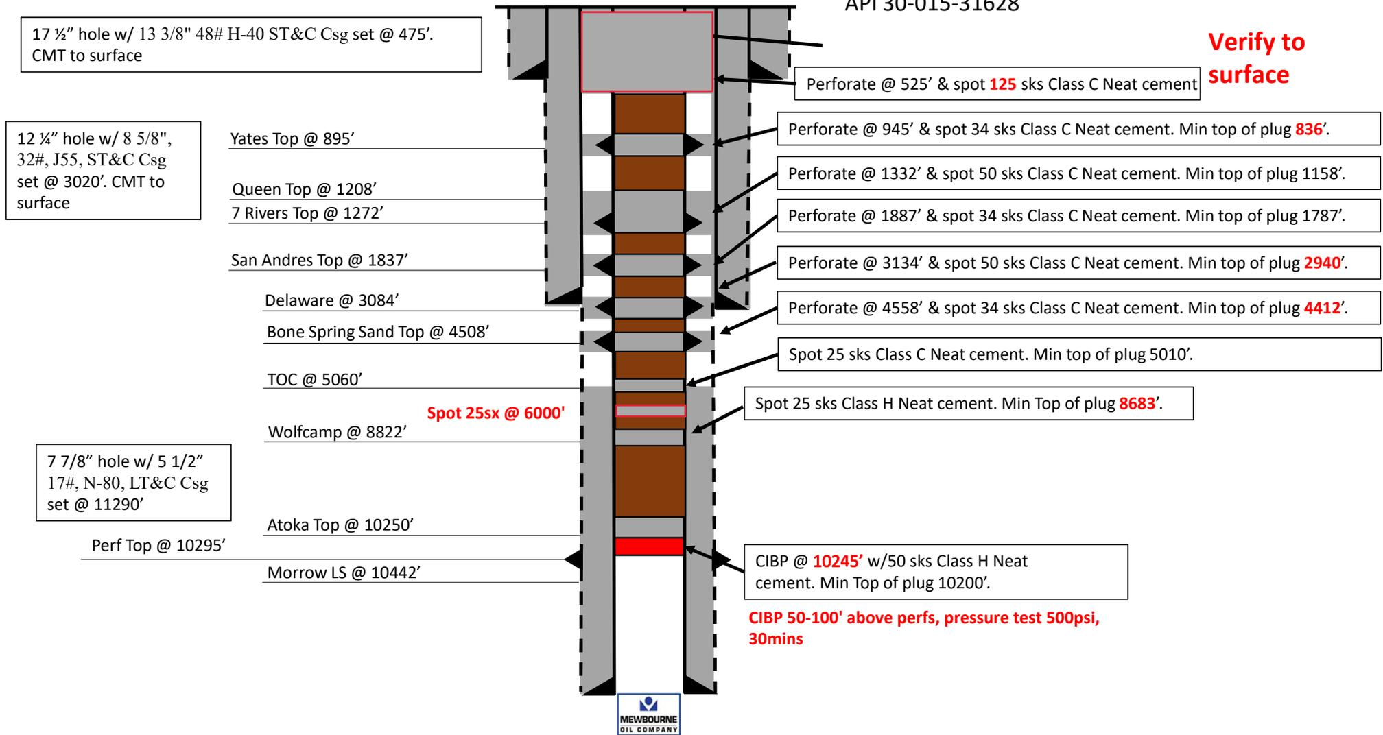
BLM Edits: 10% excess per 1000' by length for plug tops. High cave karst => 500' surface plug. Spacer plug at 6000' to avoid >3000' between plugs. Leak test CIBP 500psi, 30mins. Place CIBP 50-100' above perfs
