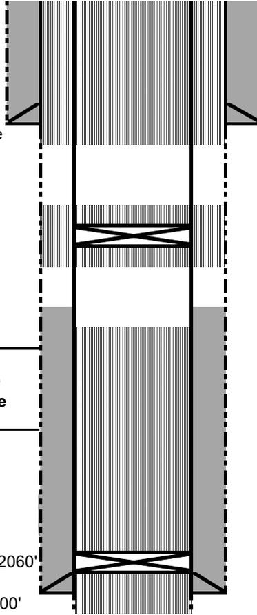
**Plug 4: Surface casing shoe, surface: Perf holes at 183'. Mix and pump sufficient cement to bring TOC to surface, inside and outside.**
