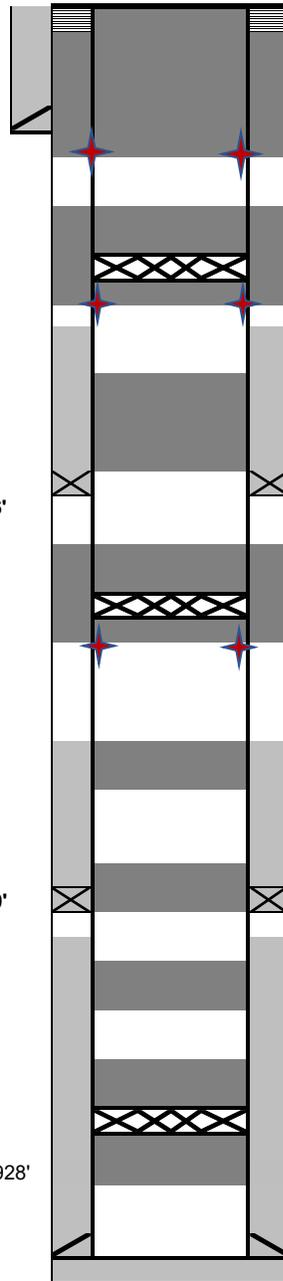
10-17-2022: TOC in casing at 2', cut off WH, TOC in 8 5/8" at 9'. Install P&A marker, top off with 18 sx.
