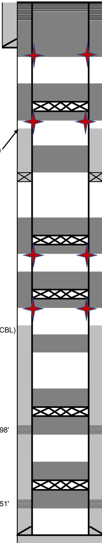
10-27-2022: Cut off WH. TOCs; 90' in annulus and 25' in casing. Install P&A marker, top off with 35 sx.
