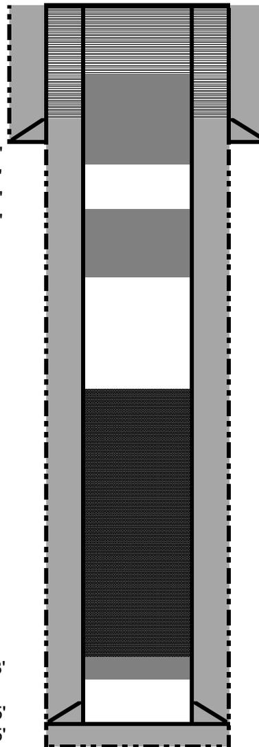
9-12-2022: Cut off WH, TOCs at 120' in annulus and 48' in casing. Install P&A marker. Top off with 38 sx.
