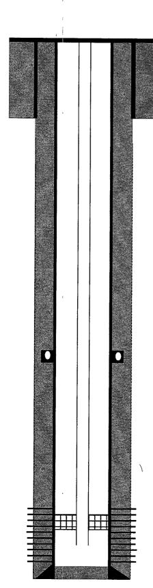
8-5/8" J-55 24# casing @ 228'. Cemented with 180 sks, 212 cf Class B w/ 3% CaCl2. Circulated 5 bbls to surface. Hole size: 12-1/4
