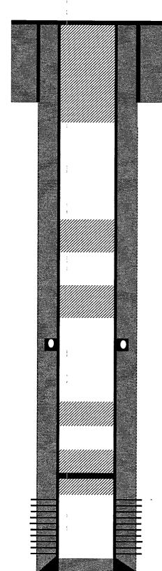
8-5/8" J-55 24# casing @ 228'. Cemented with 180 sks, 212 cf Class B w/ 3% CaCl2. Circulated 5 bbls to surface. Hole size: 12-1/4
