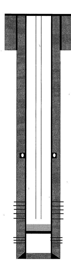
8-5/8" J-55 24# casing @ 354'. Cemented with 250 sks, Type 5 cement w/ 3% CaCl2. Circulated 18 bbls cement to surface. Hole size: 12-1/4
