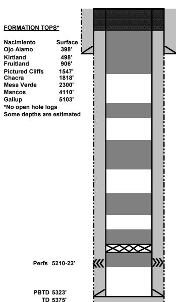
3-18-2022: Cut off WH. TOC; casing at 93', annulus at 100'. Install P&A marker. Top off casing and annulus with poly pipe and 50 sx.
