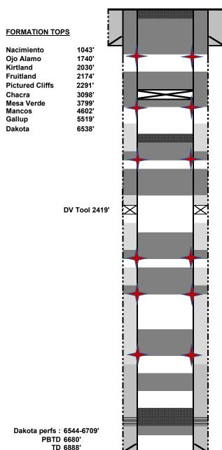
4-22-2022: Cut off WH. Install P&A marker, TOCs at surf in annulus and 8' in 3 1/2" csg. Top off csg and cellar with 31 sx.
