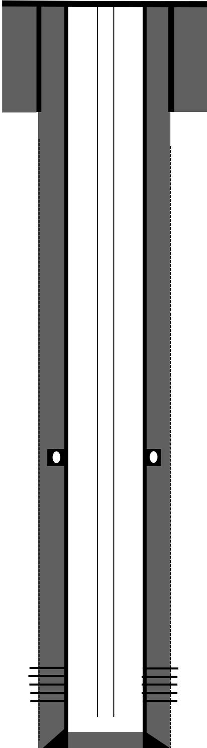
8-5/8" 24# casing @ 312'. Cemented with 211 sks, Class B cement w/ 2% CaCl<sub>2</sub>. Circulated cement to surface. Hole size: 12-1/4
