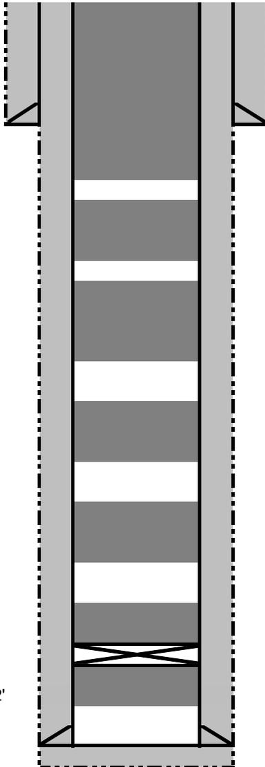
**Plug 7: (Ojo Alamo, surface casing shoe, and surface plugs): Spot balanced plug from 313' to surface. Top off casing as necessary.**
