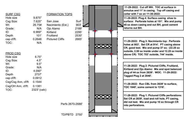
All cement used Type II/V mixed at 15.0 ppg, yirld 1.29 cuft/sx Regulatory representative: Wanda Weatherford, BLM and Monica Kuehling, NMOCD via phone GPS Coordinates; Lat 36.2425385 N, Long 107.2737409 W
