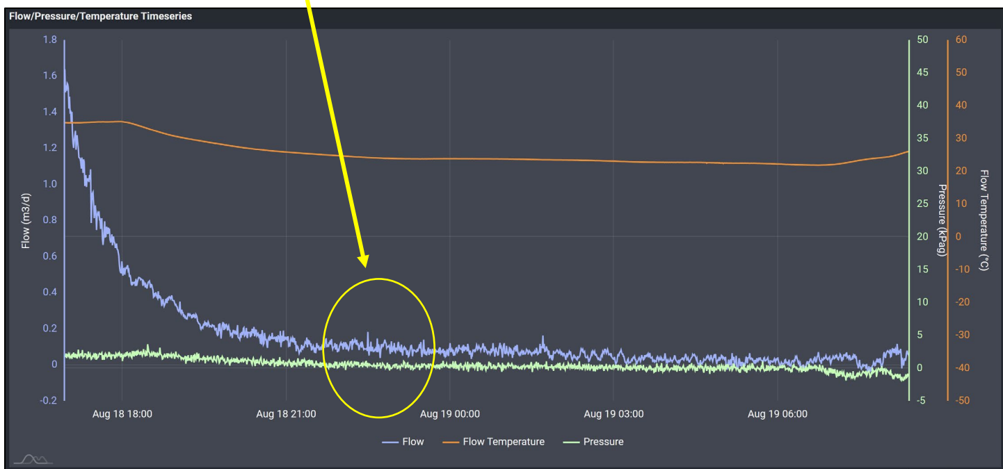
Image 4.2 – TLSA #030 (30-005-60595) Methane Flow/Pressure/Temperature Timeseries & Peak Flow for entire testing period or 15.5-hours.
