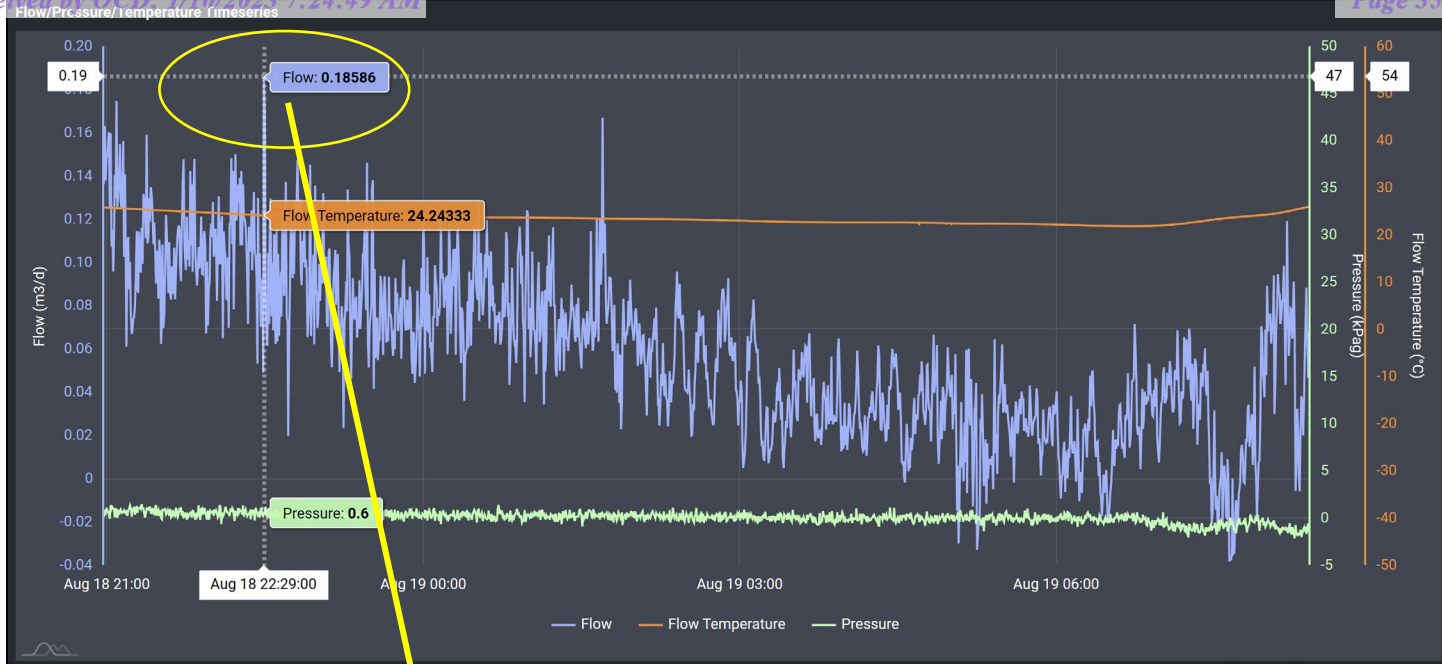
Image 4.1 – TLSA #030 (30-005-60595) Methane Flow/Pressure/Temperature Timeseries & Peak Flow at Interval #1 testing period of 11.4-hours.
