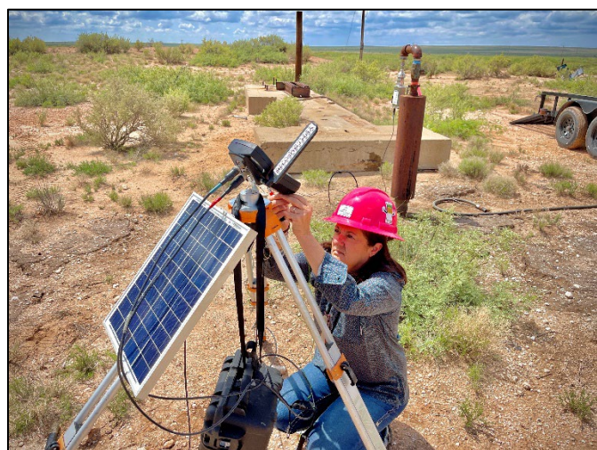
3) TLSA #030 (30-005-60595) – Methane Flow Test Rig Up
