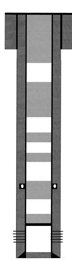
8-5/8" 24# casing @ 213'. Cemented with 135 sks, Class B cement w/ 2% CaCl2 (159 Cu.ft). Circulated cement to surface. Hole size: 12-1/4
