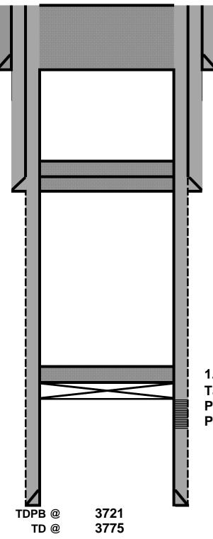
13 3/8 CSG @ 220 4. Perf'd @ 270'. Pressured up on perfs to 500 PSI. ND BOP. Spotted 60 sx class C cmt @ 332' to surface.
