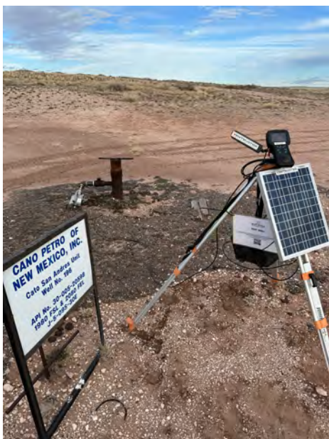
CSA #196: Methane Testing
