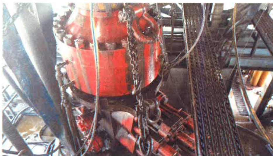
Figure 1: Winch System attached to BOP Stack
