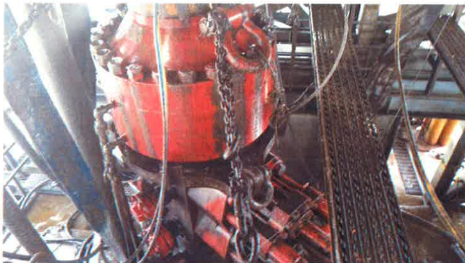
Figure 1: Winch System attached to BOP Stack
