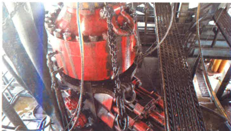
Figure 1: Winch System attached to BOP Stack
