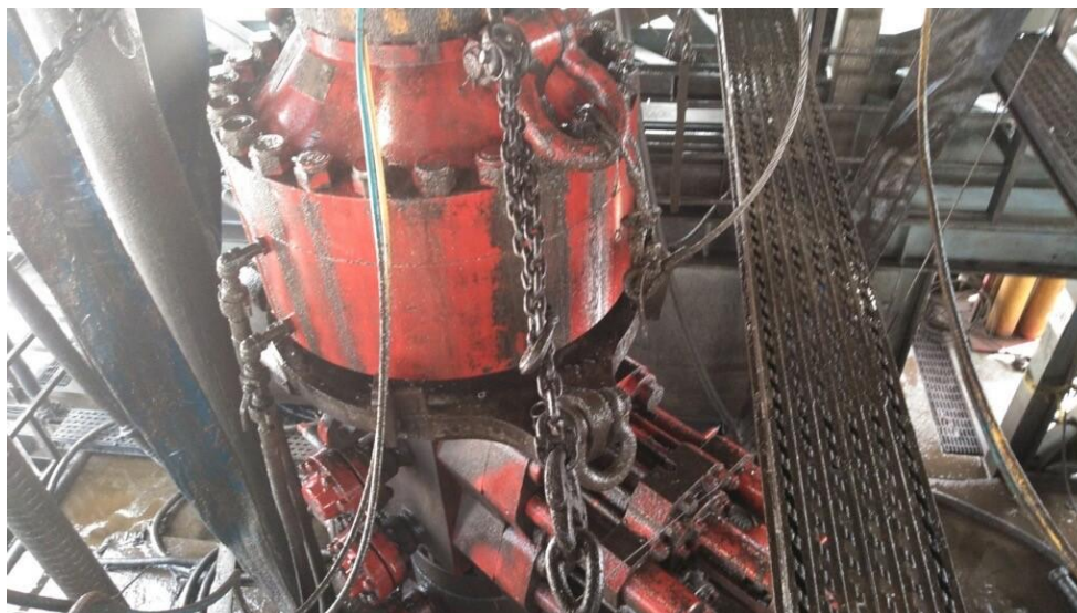
Figure 1: Winch System attached to BOP Stack
