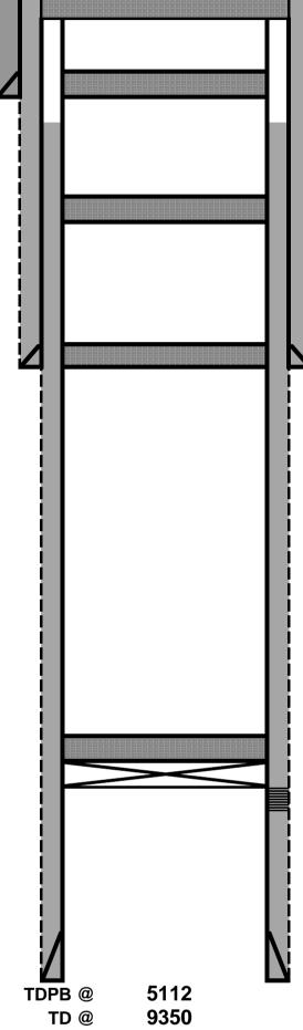
5. Perf'd @ 200'. Pressured up on perfs to 500 PSI. Spotted 54 sx class C cmt @ 251' & circulated to surface.
