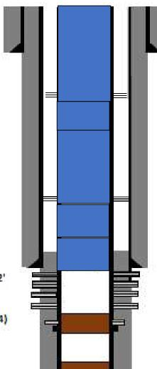
perf @ 1915' - squeeze 500 sx class C cmt from 1920' - 0' Cement to Surface.
