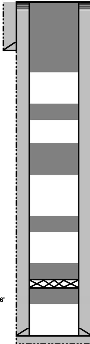
2-3-2023: TOC in 5 1/2" casing at surface, cut off WH, TOC at 10' in 8 5/8" surface casing. Install P&A marker. Top off cellar and casings with 34 sx.
