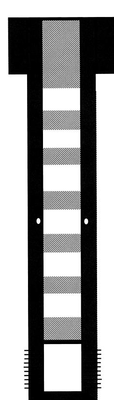
9-5/8" J-55 36# casing @ 267'. Cemented with 184 sks, 248 cf, Type III w/ 2% CaCl2. Circulated 16 bbls cement to surface. Hole size: 13-1/2"
