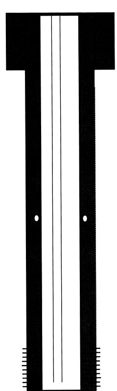
9-5/8" J-55 36# casing @ 267'. Cemented with 184 sks, 248 cf, Type III w/ 2% CaCl2. Circulated 16 bbls cement to surface. Hole size: 13-1/2"
