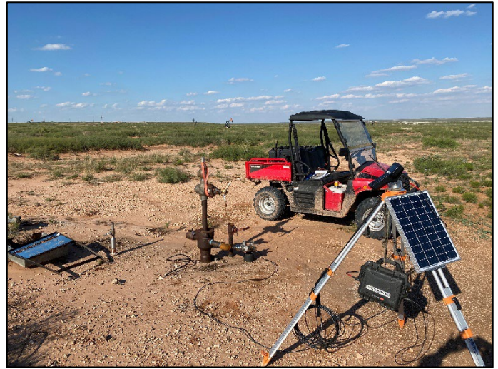
2) TLSA #78K (30-005-60995) – Methane Monitoring Rig Up
