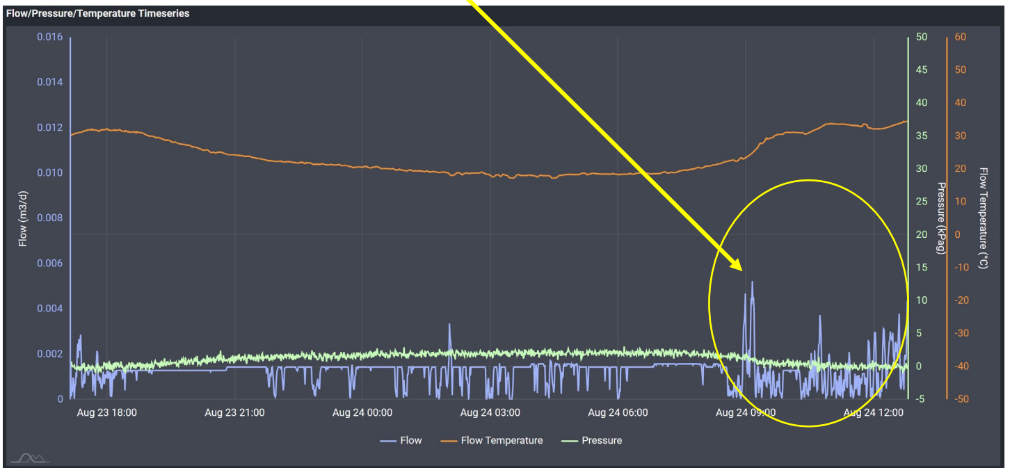
Image 4.2 – TLSA #78K (30-005-60995) Methane Flow/Pressure/Temperature Timeseries & Peak Flow for entire testing period or 19.75-hours.
