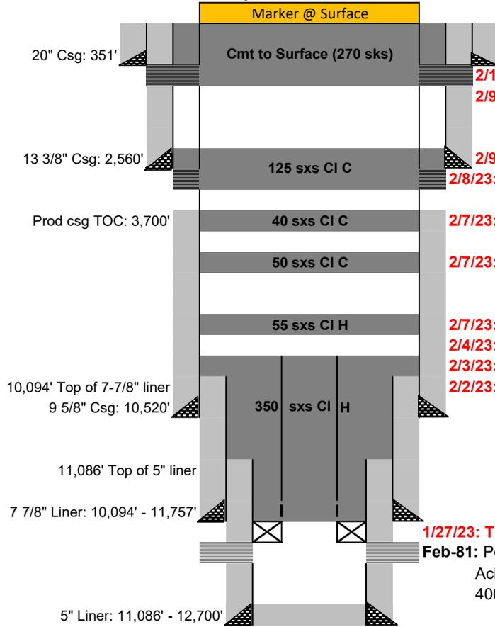
**2/15/23: Cut & removed wellhead; Topped off and verified cement to surface on all strings; Weld on dryhole marker & riser; filled cellar and back drug location.**
