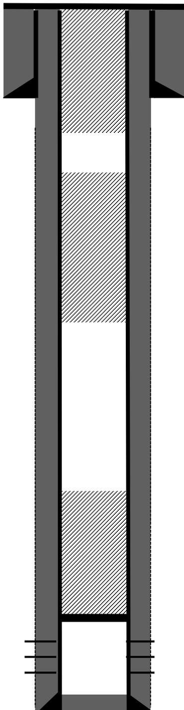
8-5/8" 24# casing @ 280'. Cemented with 180 sks Class B cement w/2% CaCl<sub>2</sub>. Hole size: 12 1/4". Circulate 15 bbls cement to surface.
