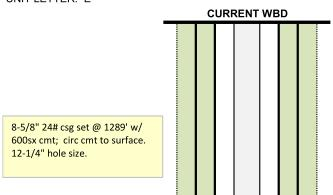
4-1/2" 10.5# csg set @ 3392' w/ 750sx cmt; circ cmt to surface. 7-7/8" hole size.
