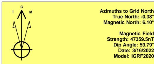
To convert a Magnetic Direction to a Grid Direction, Add 6.10°
