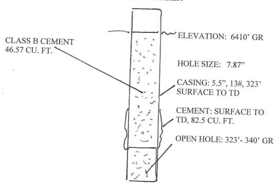
SFP 103 WELLBORE DIAGRAM 30-031-20063 165' FSL AND 165' FEL P, SEC. 21, T20N, R9W
