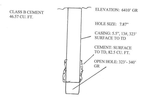
5/10/2023 REMOVE PRODUCTION EQUIPMENT, CIRCULATE WELLBORE, 5/12/2023 FILL WELLBORE FROM TD TO SURFACE WITH 46.57 CU. FT. CLASS B CEMENT,
