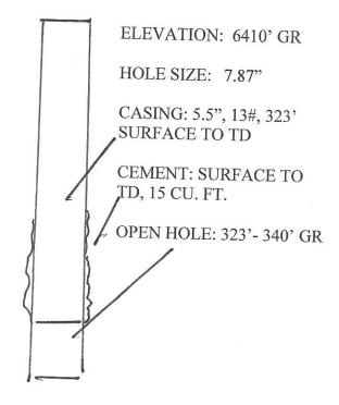
4/20/2023 REMOVE PRODUCTION EQUIPMENT, CIRCULATE WELLBORE, 4/21/2023 FILL WELLBORE FROM TD TO SURFACE WITH 46.57 CU. FT. CLASS B CEMENT, 4/23/2023 PLACE DRY HOLE MARKER, CLEAN AND RECLAME LOCATION OF APPROXIMATELY 1000 SQ. FT.
