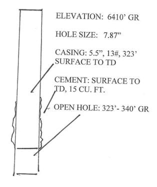
4/20/2023 REMOVE PRODUCTION EQUIPMENT, CIRCULATE WELLBORE, 4/21/2023 FILL WELLBORE FROM TD TO SURFACE WITH 46.57 CU. FT. CLASS B CEMENT, 4/23/2023 PLACE DRY HOLE MARKER, CLEAN AND RECLAME LOCATION OF APPROXIMATELY 1000 SQ. FT.
