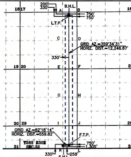
Diagram details: B.H.L. (Bottom Hole Location) at grid AZ = 359°34'31", HORIZ. DIST. = 12,246.67'. S.H.L. (Surface Hole Location) at grid AZ = 82°18'14", HORIZ. DIST. = 559.82'. Distances from surface to bottom hole: 750' (North), 750' (East), 330' (South), 258' (West).
