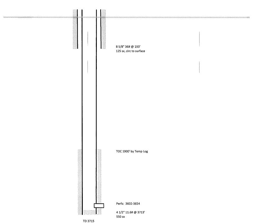
Operataor: Trigg Oil and Gas Well Name NE SQ Lake 18 API # 30-015-04832 Location: Sec 9, T16S, R31E Date Spud 7-12-1960 Date Complete 9-6-1960
