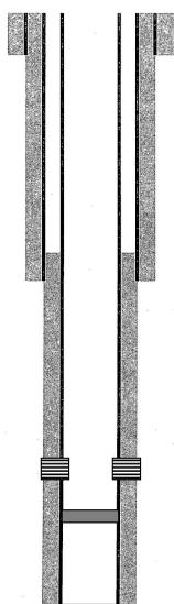
17-1/2" hole @ 855' 13-3/8" csg @ 855' w/ 725sx-TOC-Surf-Circ
