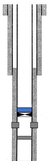
17-1/2" hole @ 855' 13-3/8" csg @ 855' w/ 725sx-TOC-Surf-Circ
