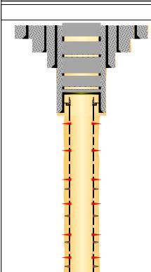
Cement; 0.0-100.0 ftKB Conductor; 24 in; 118.0 ftKB
