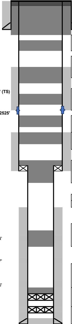
Top off Plug: Cut off WH, install subsurface P&A marker, top off casings and cellar as needed.
