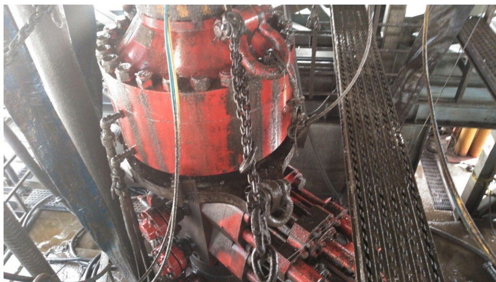
Figure 1: Winch System attached to BOP Stack
