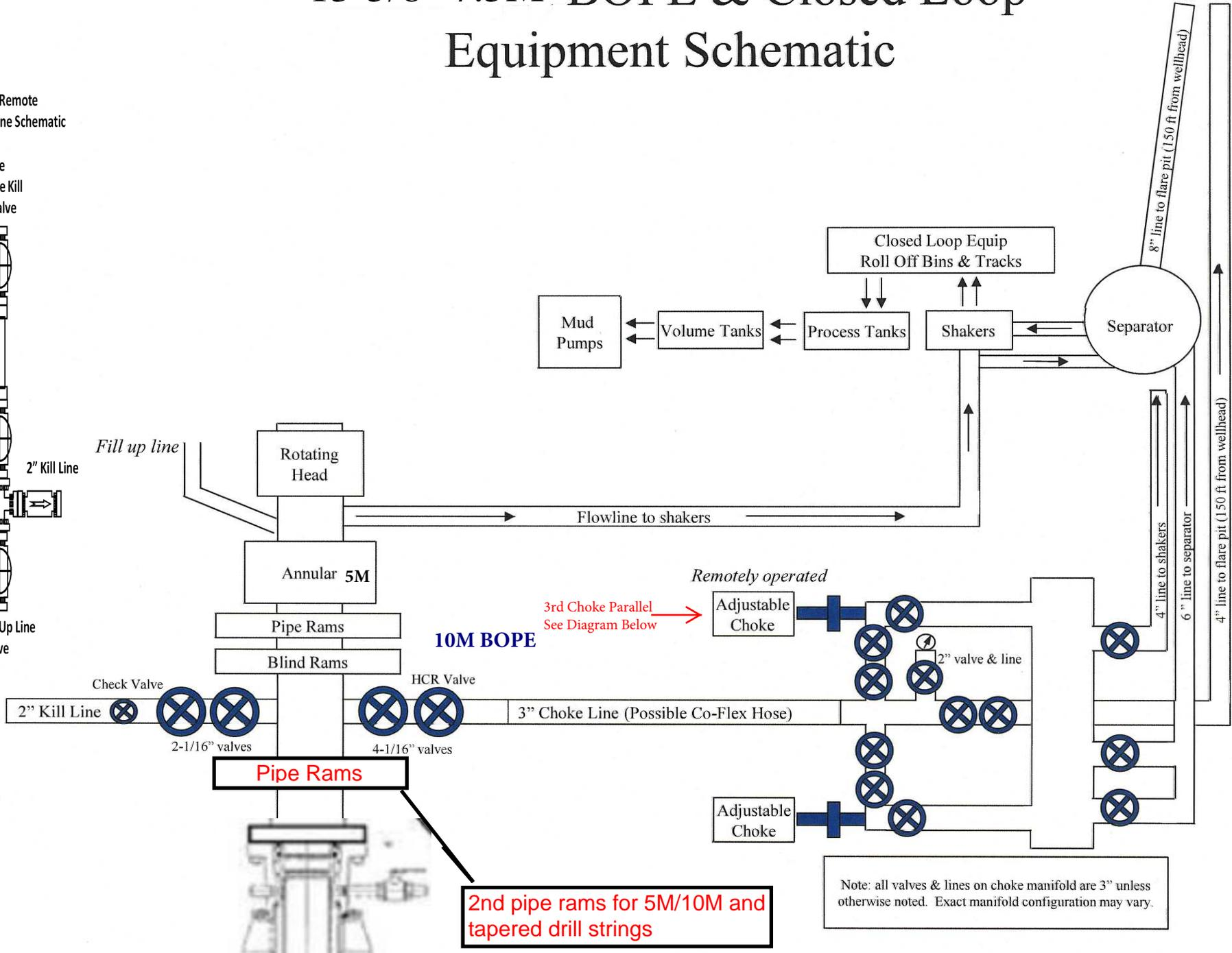
Note: all valves & lines on choke manifold are 3" unless otherwise noted. Exact manifold configuration may vary.
