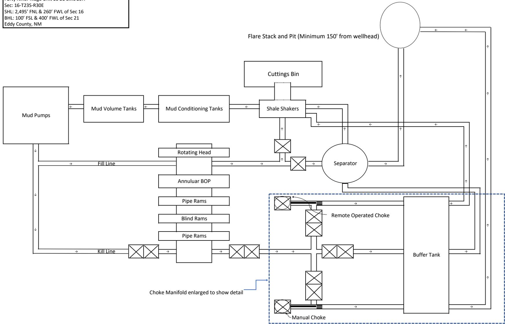
Choke Manifold enlarged to show detail
