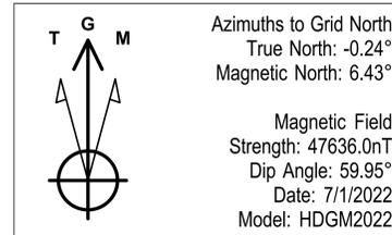
To convert a Magnetic Direction to a Grid Direction, Add 6.432°
