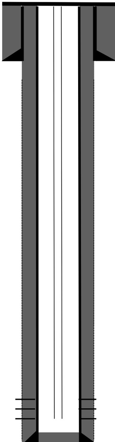
7" 20# casing @ 128'. Cemented with 65 sks Class B cement.
