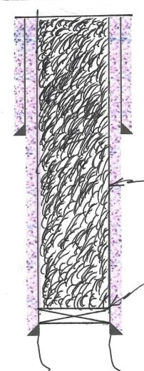
9-5/8" 36 # CASING SET @ 284' IN 12-1/2" HOLE. CEMENT CIRCULATED TO SURFACE W/140 Sks.
