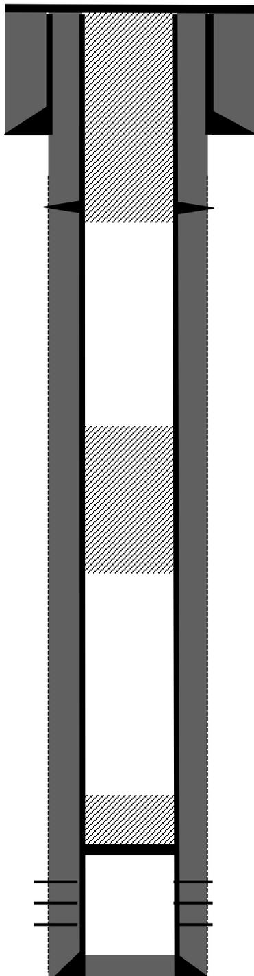
7" 20# casing @ 127'. Cemented with 65 sks Type 5 cement.
