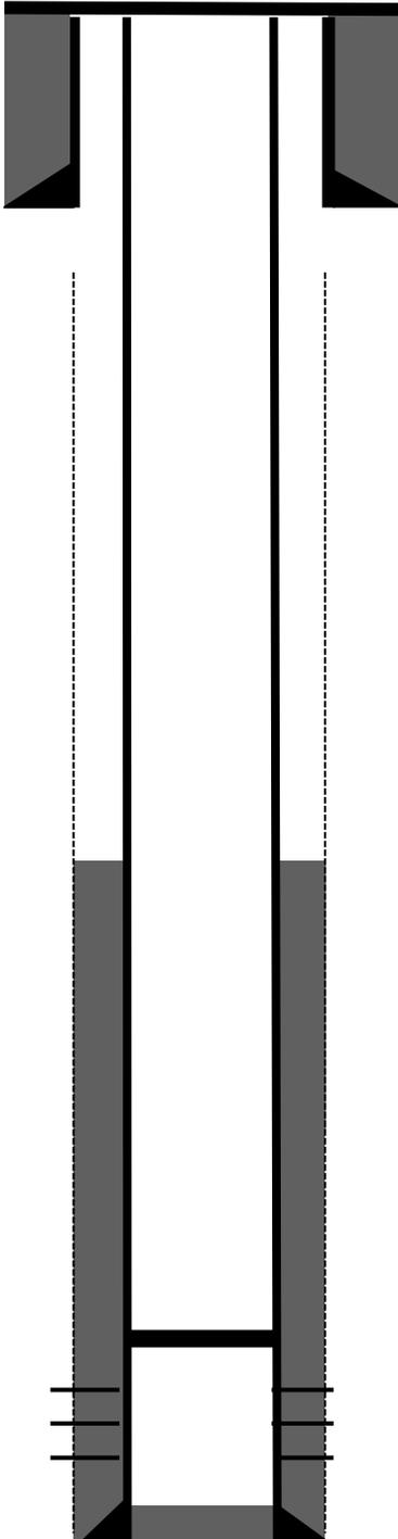
7" 20# casing @ 139'. Cemented with 65 sks Type 5 cement.
