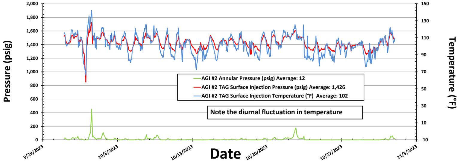
**FIGURE #7: LINAM AGI #2 TAG INJECTION PRESSURE AND CASING ANNULAR PRESSURE DIFFERENTIAL (PSIG)**
