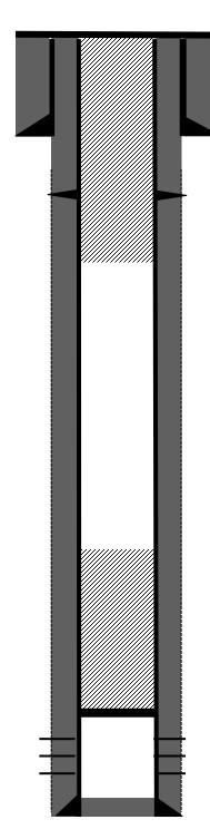
8-5/8" 24# casing @ 132'. Cemented with 95 sks Class B cement. Hole size: 12-1/4". Circulate 7 bbls cement to surface.
