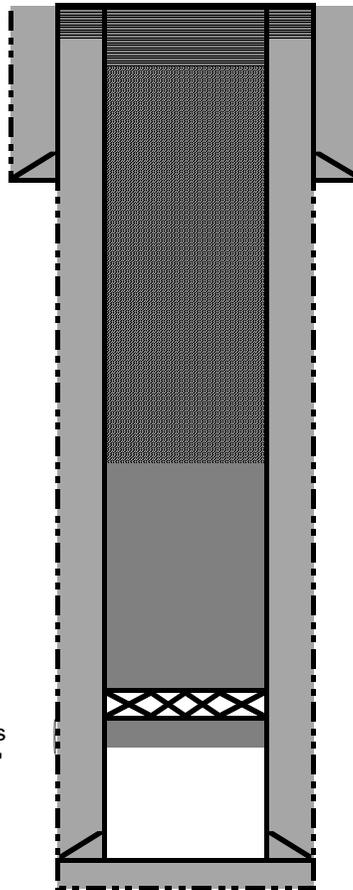
12-1-2023: Cut off WH, TOC in 7" casing at 28'. Install P&A marker. Top off casings and cellar with 28 sx.
