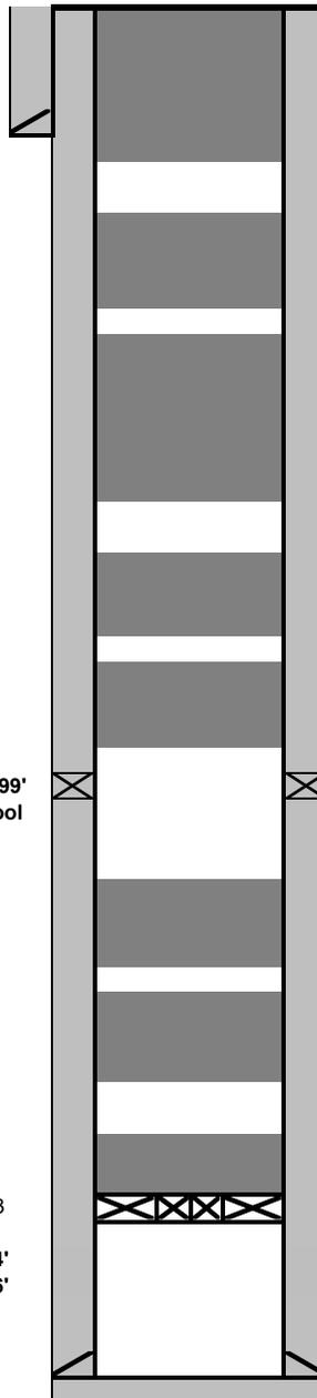
**Plug 8:** Surface casing shoe to surface: Mix and spot balanced plug from 601' to surface. Cut off WH, install P&A marker
