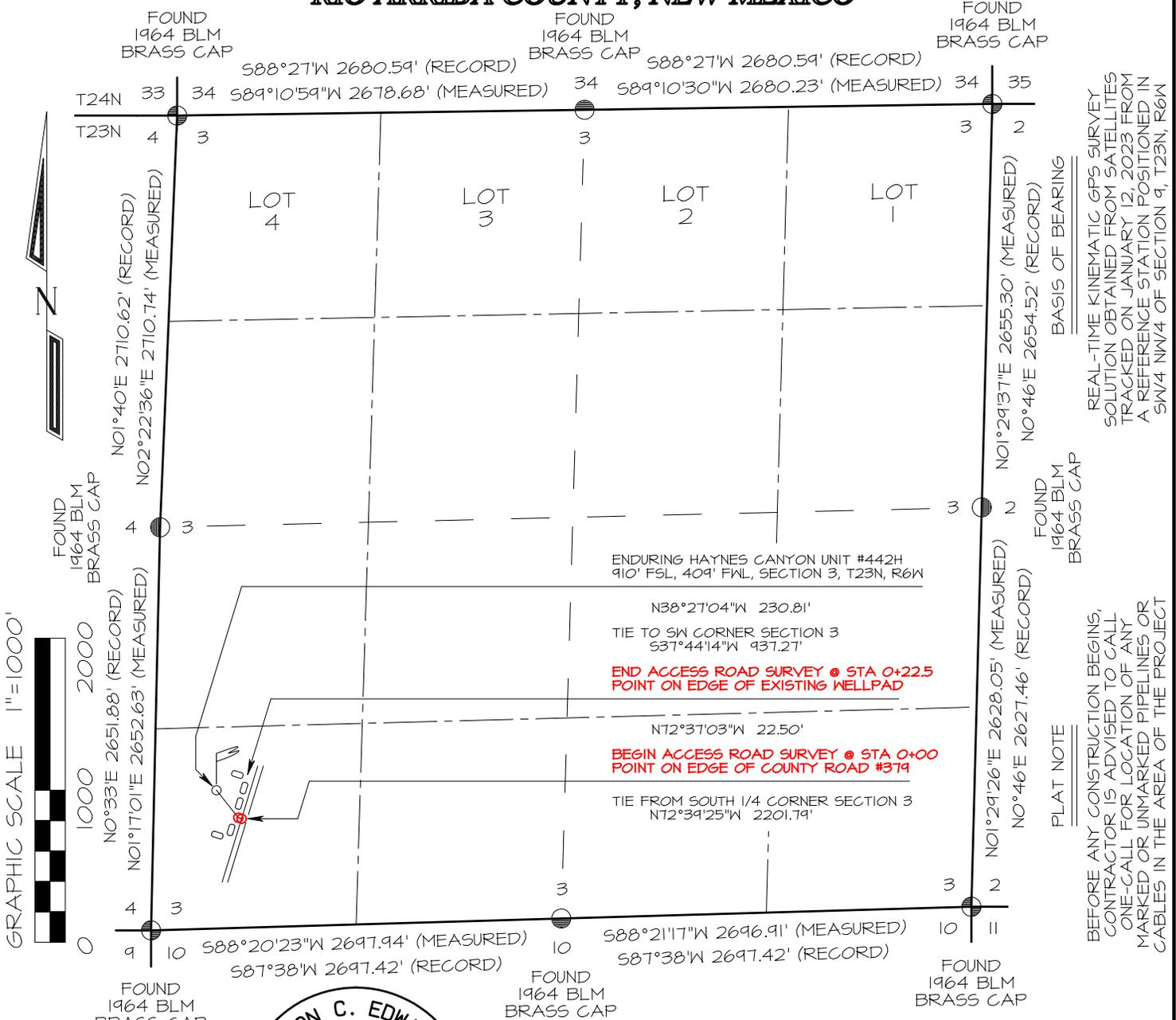
REAL-TIME KINEMATIC GPS SURVEY SOLUTION OBTAINED FROM SATELLITES TRACKED ON JANUARY 12, 2023 FROM A REFERENCE STATION POSITIONED IN SW/4 NW/4 OF SECTION 9, T23N, R6W
