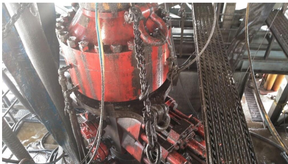
Figure 1: Winch System attached to BOP Stack
